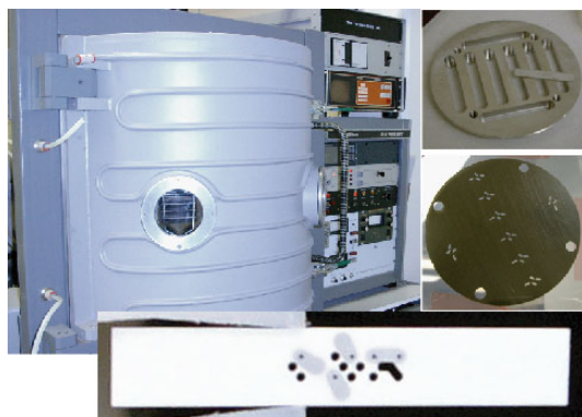
Figure 7: Contacts are evaporated onto the base substrates through photomasks using physical vapor deposition (PVD).
