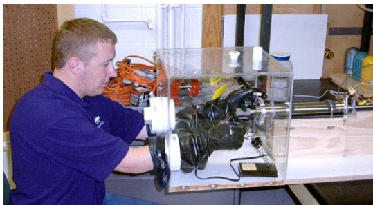
Figure 8: Custom glove box designed for backfilling the detectors with argon fill gas.
