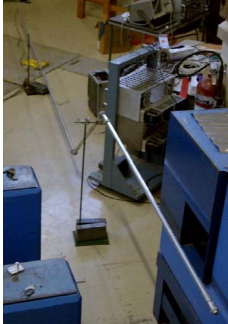
Figure 21: Tube for in-core testing of an MPFD. Here it is being tested in the beam port prior to insertion into the reactor.
