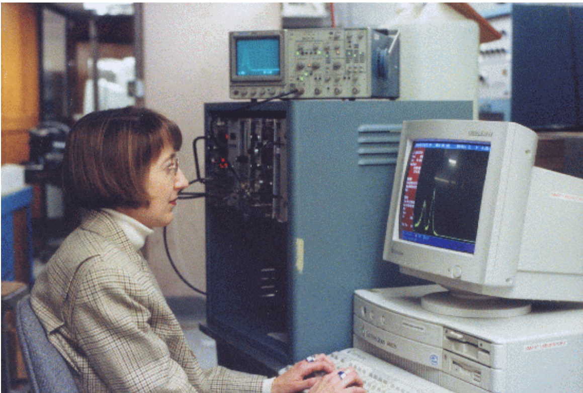
Figure 2: Holly Gersch, a Nuclear Engineering graduate student, operates a ^{10}\text{B} -coated self-biased GaAs detector at nuclear reactor neutron beam port. The detector functions without an applied voltage. The two major ^{10}\text{B}(n,\alpha)^7\text{Li} reaction product energy peaks show up clearly on the multi-channel analyzer computer screen.
