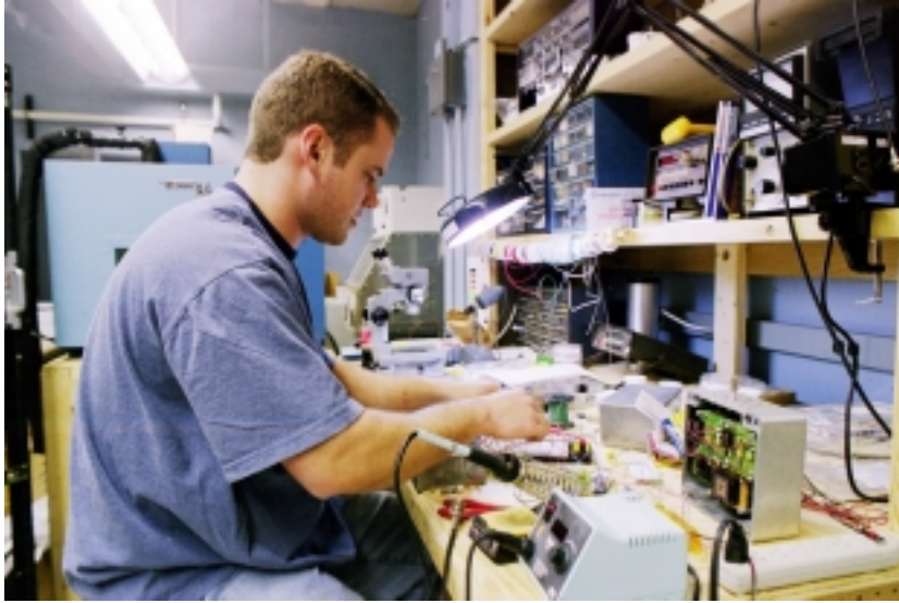
Figure 1: Jeff Sanders, a Nuclear Engineering graduate student, puts the finishing touches on the electronic circuitry for a radiation-hardened bulk GaAs neutron-imaging array (lower right). The GaAs neutron imaging chip and electronics was later placed in a radiation hot cave to measure the neutron sensitivity from epithermal neutron sources.
