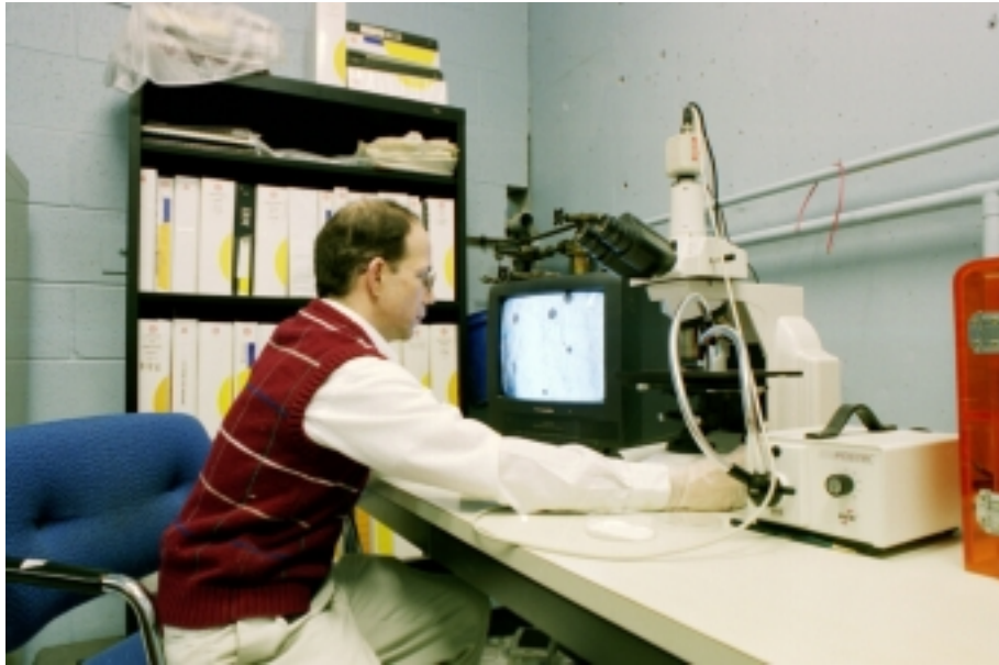
Figure 2: Dr. McGregor carefully inspects a CdZnTe sample for crystal defects and imperfections with an infrared microscope. Cracks and major defects will cause the CdZnTe devices to perform poorly. The crystals are etched, inspected, and mapped before pieces are cut for device fabrication.
